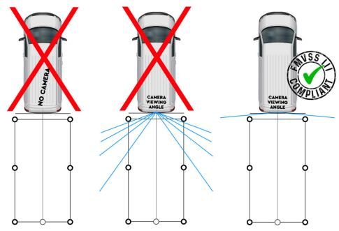
**NOTE:** Camera must be installed flush between 5"-96" off the ground and in a range of 12" in either direction from the center of the vehicle (at the 40"-50" height) in order to be compliant with FMVSS 111.
